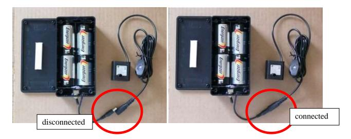
Here the pump being connected to the transformer (the pump is in the bowl, you only see the cord and on/off switch). It can be plugged into an electrical outlet now.
